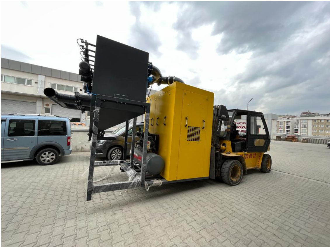
Blower System with 8,000 m 3 /h Capacity
